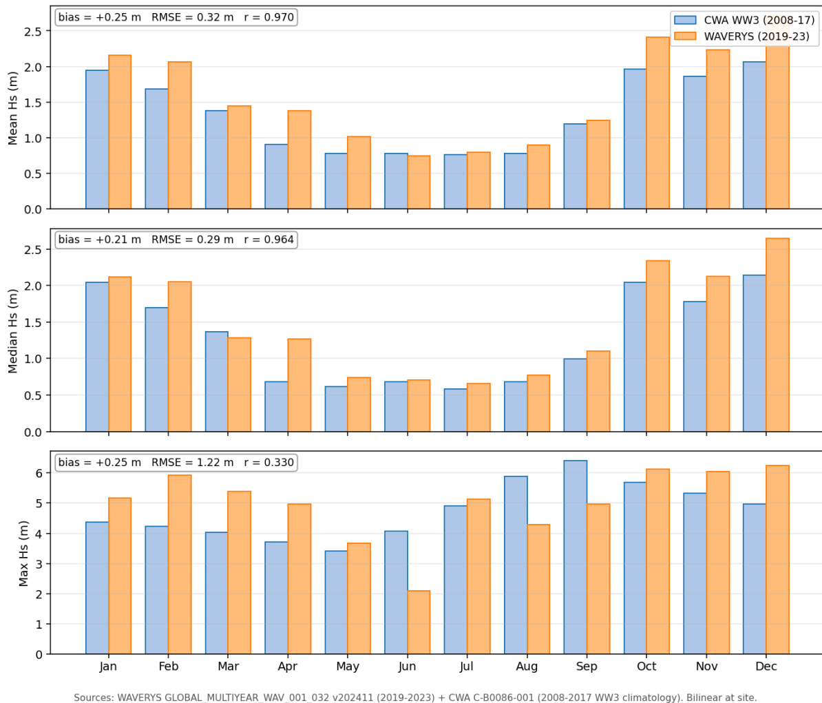
Figure 9: Monthly Hs comparison at site: WAVERYYS 5-yr (2019-2023) vs CWA WW3 10-yr (2008-2017). Panels show mean / median / max with bias, RMSE, and Pearson r.
