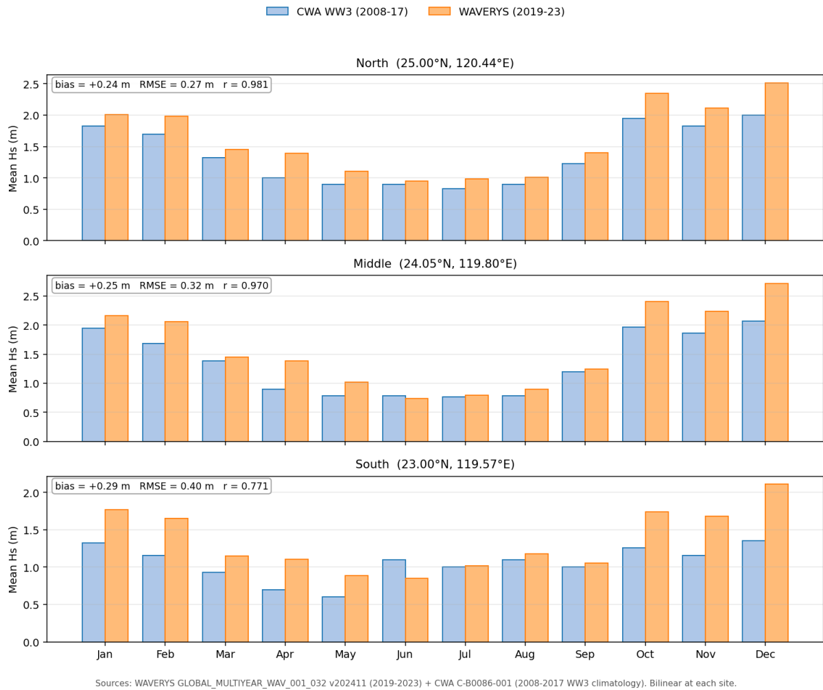
Figure 10: Per-site monthly mean Hs cross-check: WAVERYYS multiyear reanalysis (2019-2023, orange) vs CWA WW3 climatology (2008-2017, blue), bilinear-interpolated at each of the three study sites. Top: North (25.00°N, 120.44°E); middle: Middle (24.05°N, 119.80°E); bottom: South (23.00°N, 119.57°E). Per-panel stats box: bias, RMSE, Pearson r over the 12-month seasonal cycle. WAVERYYS reads systematically higher than CWA WW3 at all three sites (~0.25 m bias), with seasonal-cycle Pearson r \geq 0.97 at North and Middle and r = 0.77 at South.
